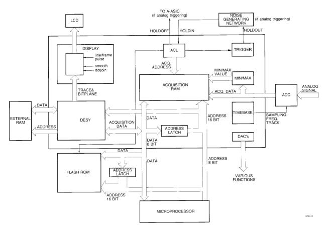
Figure 3.3 Schematic Diagram D-ASIC D1203
